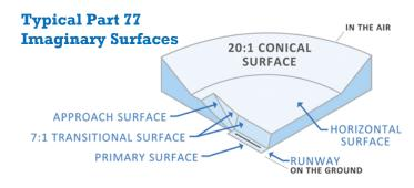
**Height Notification Requirements:** The graphics below illustrate the typical notification requirements associated with building in proximity to CLE and BKL. Note that requirements associated with other airports in the Cleveland area may be applicable.
