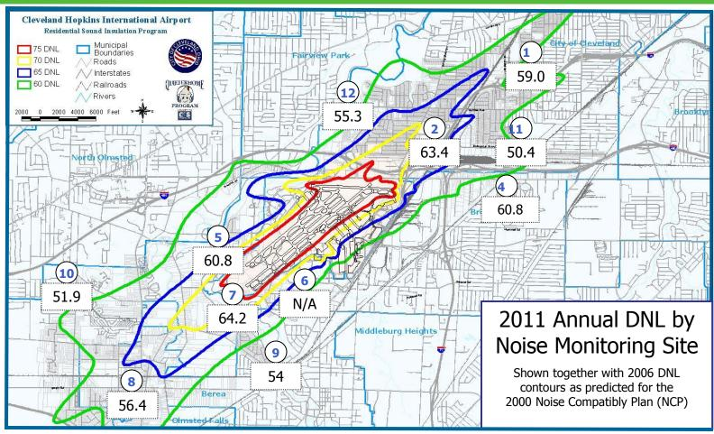
Due to outages and malfunctions, the DNL calculations for NMS01, 02, 04, 05, 07, 08, 10, 11 and 12 were based on the following number of days respectively 364, 315, 305, 354, 365, 349, 332, and 352 days. NMS09 had 44 days of data, mostly from Jan and Feb, and its DNL was estimated from flight data.
