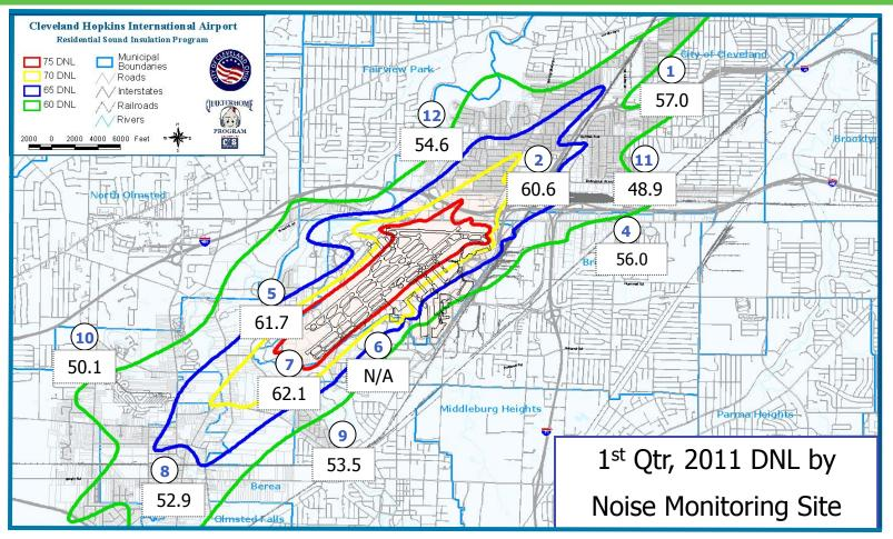
Due to malfunctions at NMS09 in Feb and Mar, the quarterly DNL at NMS09 was estimated from daily Jan DNLs and the runway use patterns over the remainder of the quarter. NMS06 was disconnected from power, dismantled and placed in storage in November 2008 due to runway expansion. 6 Noise Compatibility
